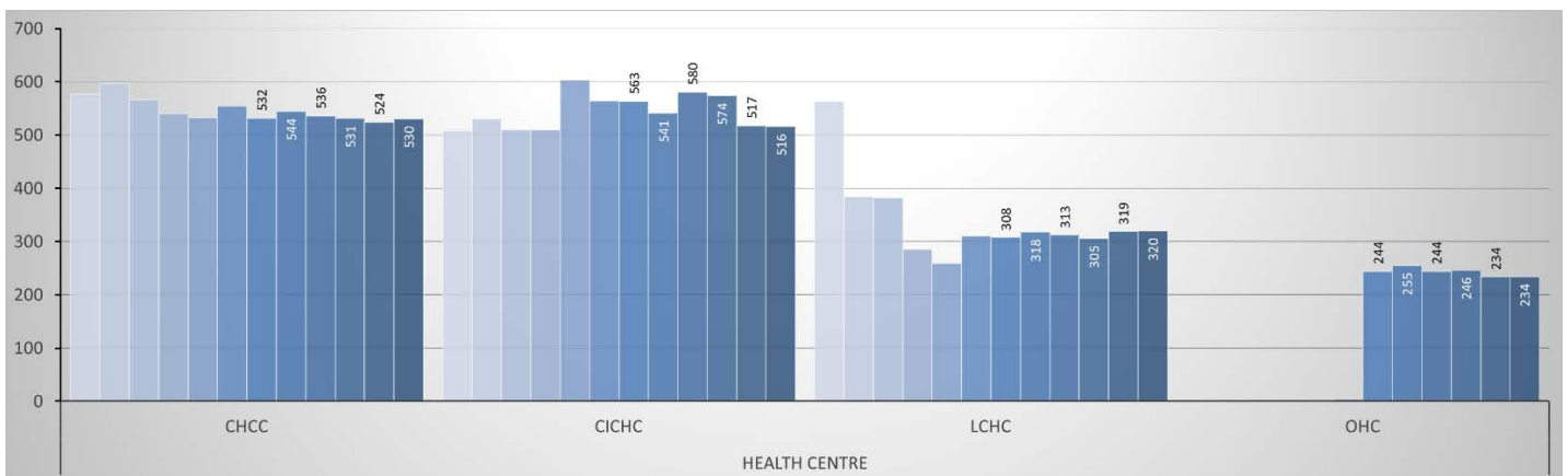
Figure 10. Health Centre F2008 to F2019 EUI Performance (kWh/m 2 )
